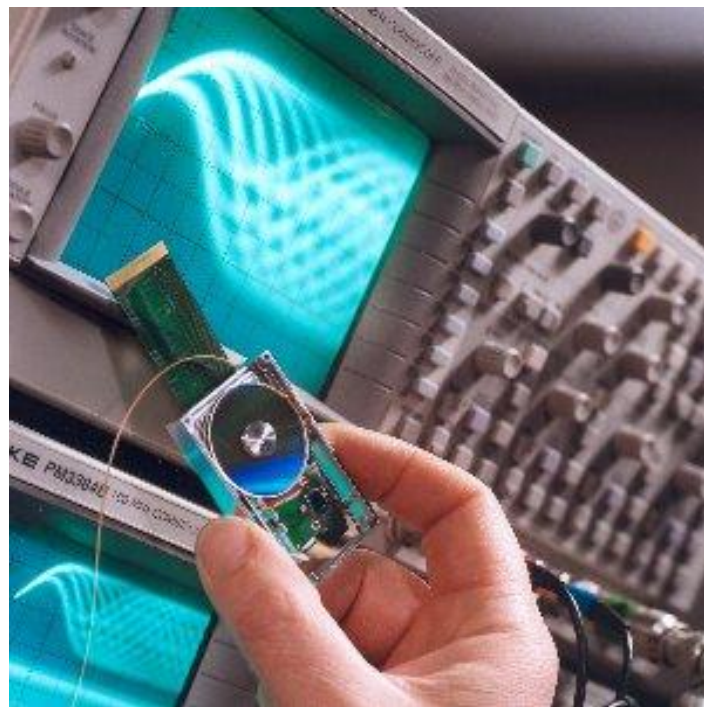
Figure Z1-2 Philips prototype blue micro-optical disc system.
